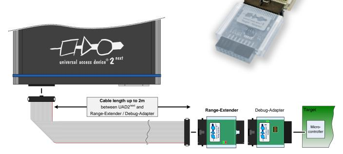
The **Universal Debug Engine® (UDE)** is a powerful development platform for debugging, testing and system analysis of microcontroller software applications. The UAD2<sup>pro</sup>, UAD2<sup>next</sup> and UAD3+ access devices of the **Universal Access Device (UAD)** family complete the comprehensive debug functions of UDE and enable fast, robust and flexible communication with the target system.
