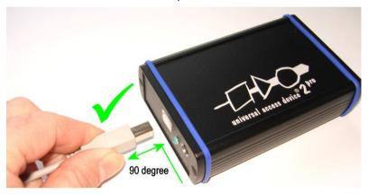
Do not insert or remove a USB plug with excessive force.
